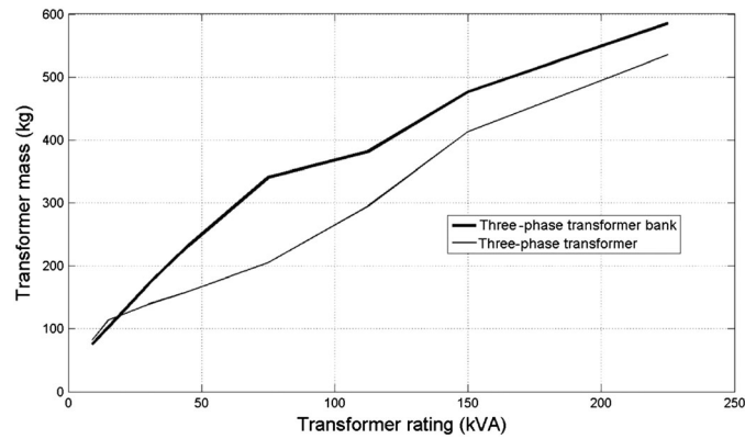
Figure 9. Weight comparison between three-phase transformers and three-phase transformer banks (transformer manufacturer 0).
